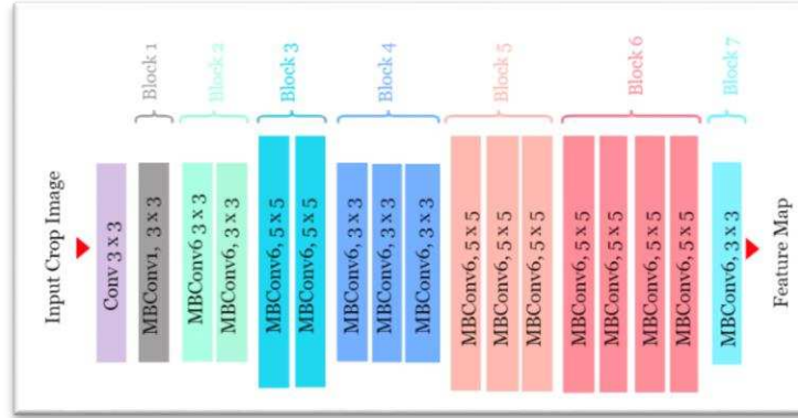
1-Figure 3.4 Detailed of the EfficientNetB0 architecture [16].
