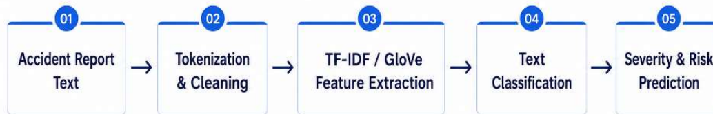
Figure 2.10: NLP pipeline for accident report analysis.
