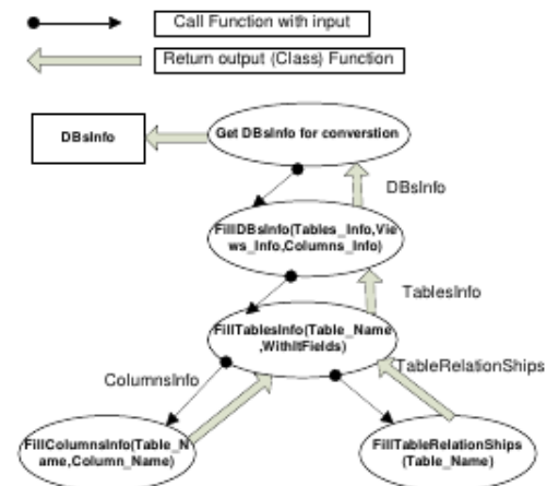
Figure 1: Processor of algorithms for extracting RDB metadata (DBsInfo)
