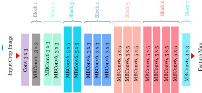
Figure 3.4 Detailed of the EfficientNetB0 architecture [16].
