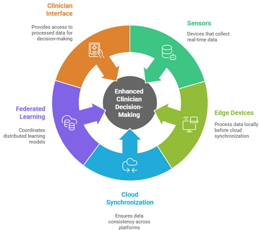
Figure 4.1: Edge-Cloud System Architecture for Diabetic Monitoring
