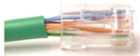
Poorly terminated UTP cable
