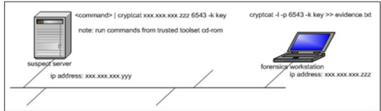
Figure 2: Volatile data collection setup
