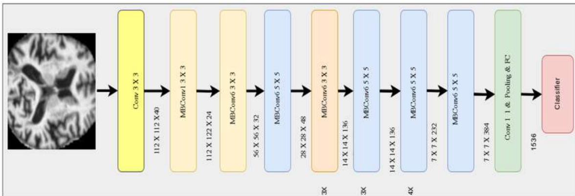
Figure 3.5: Efficient Net B3 architecture
