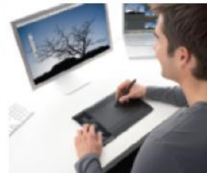
GRAPHICS/PEN TABLETS Transfer all input written or drawn on the tablet to the computer in real time and allow the use of pen flicks and other pen navigation tools.
