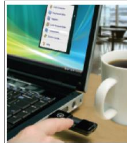
STAND-ALONE FINGERPRINT READERS Often used to control access to facilities or computer systems, such as to the notebook computer shown here.
