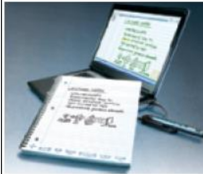
DIGITAL WRITING SYSTEMS Record all input written on the paper and transfer it wirelessly to a computer upon demand.
