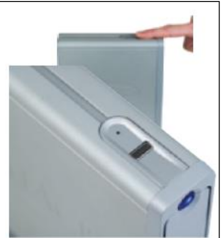
BUILT-IN FINGERPRINT READERS Typically used to control access to the device into which the reader is built, such as to the external hard drive shown here.
