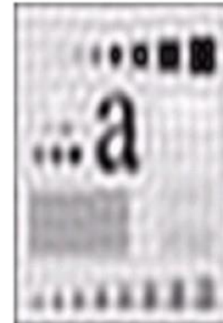
Result of filtering with ideal low pass filter of radius 15
