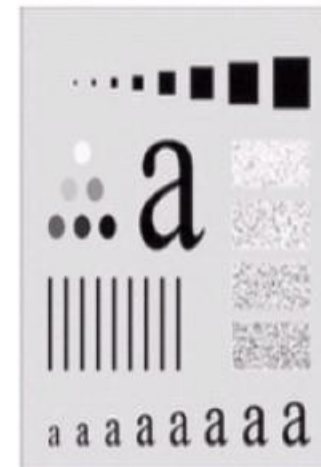
Result of filtering with ideal low pass filter of radius 80
