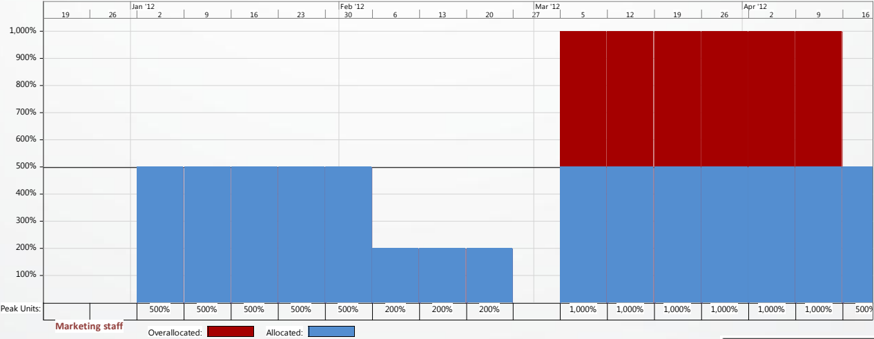
Before Leveling within Slack
