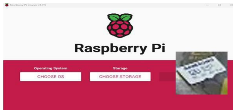
Figure 4.2 MicroSD card and Raspberry Pi Imager
