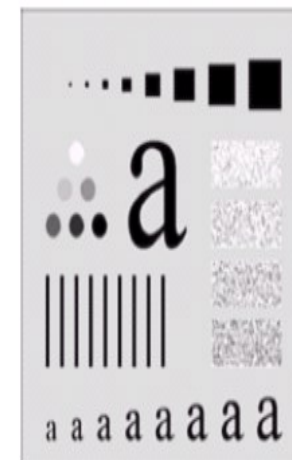
Result of filtering with Butterworth filter of order 2 and cutoff radius 80
