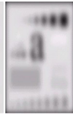
Result of filtering with Gaussian filter with cutoff radius 5
