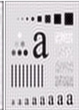
Result of filtering with ideal low pass filter of radius 30
