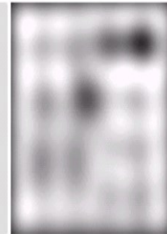
Result of filtering with ideal low pass filter of radius 5
