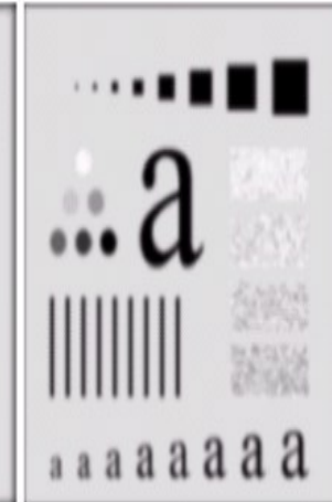
Result of filtering with Gaussian filter with cutoff radius 30
