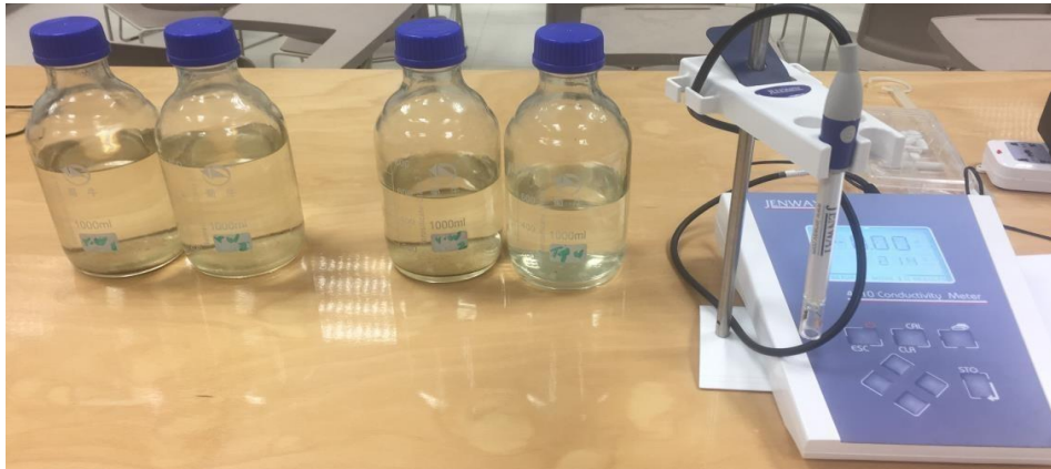
Figure 5.3: Show the device that can measure the conductivity in water (Conductivity meter) Turbidity
