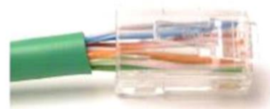
Poorly terminated UTP cable
