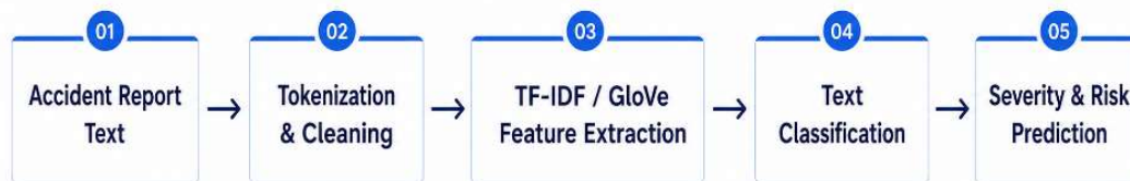
Figure 2.10: NLP pipeline for accident report analysis. Textual accident narratives are cleaned and transformed into numerical features, such as TF-IDF or word embeddings, before being used by a classifier. The figure is based on NLP accident report analysis concepts in [32] and [33].
