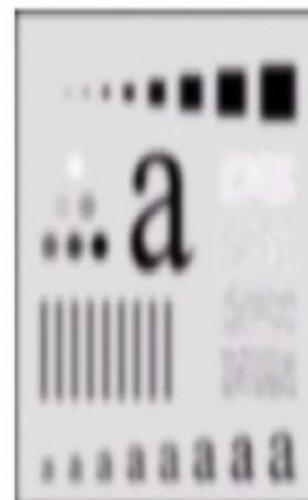
Result of filtering with Gaussian filter with cutoff radius 15
