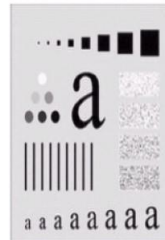
Result of filtering with ideal low pass filter of radius 80
