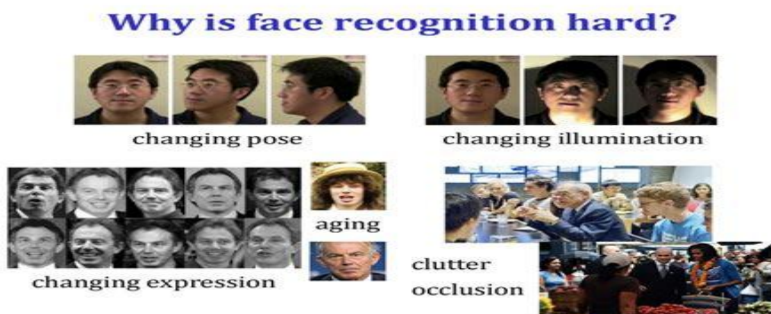
Figure 1.1: Challenges in Facial Emotion Recognition – including illumination changes, pose variations, and occlusion
