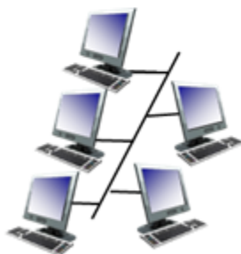
Shared Wire (e.g., cabled Ethernet)
