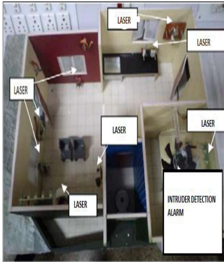
Figure 1: Surveillance system (Gobinda et al. 2014)
