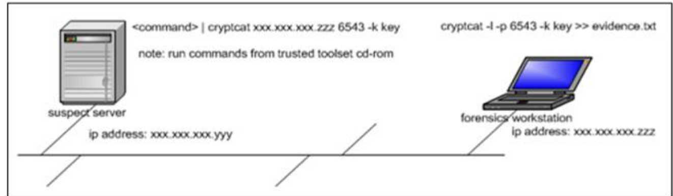
Figure 2: Volatile data collection setup
