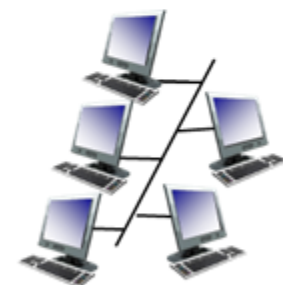
Shared Wire (e.g., cabled Ethernet)
