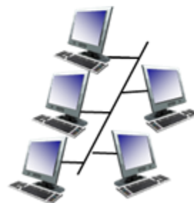
Shared Wire (e.g., cabled Ethernet)
