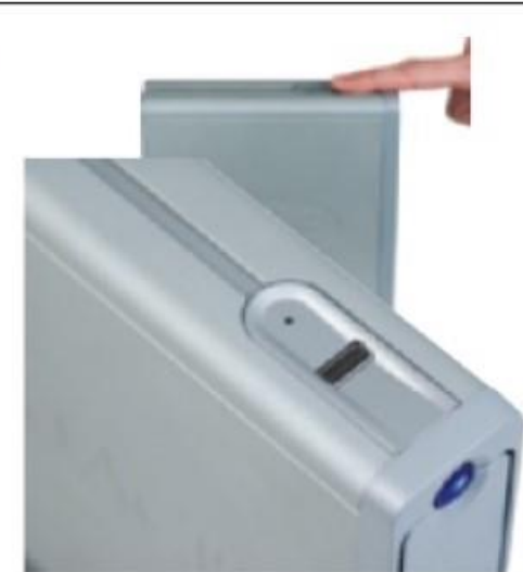
BUILT-IN FINGERPRINT READERS Typically used to control access to the device into which the reader is built, such as to the external hard drive shown here.
