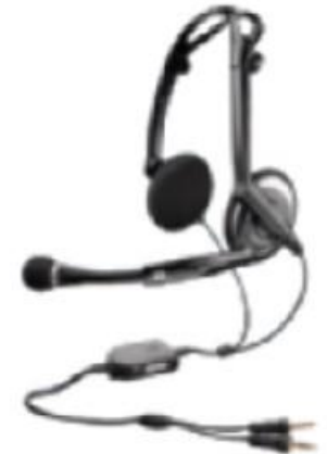
HEADSETS Used when both voice input and audio output are required.
