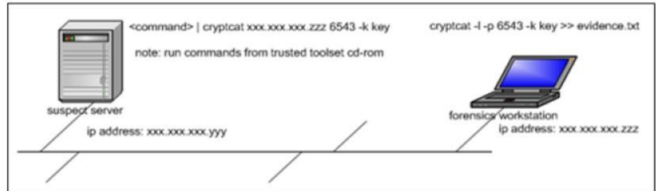
Figure 2: Volatile data collection setup
