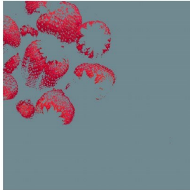
FIGURE 6.34 Color slicing transformations that detect (a) reds within an RGB cube of width W = 0.2549 centered at (0.6863, 0.1608, 0.1922) , and (b) reds within an RGB sphere of radius 0.1765 centered at the same point. Pixels outside the cube and sphere were replaced by color (0.5, 0.5, 0.5) .
